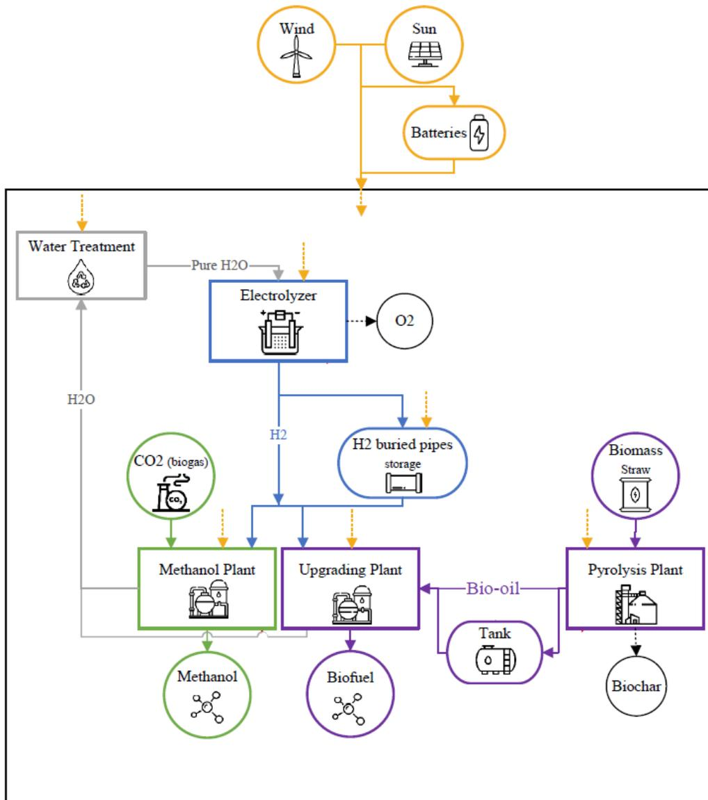
**Figure 4:** Scheme showing the behind-the-meter (BTM) power supply configuration of the Power-to-X plant and its main units considered in the model for the small-scale study.
