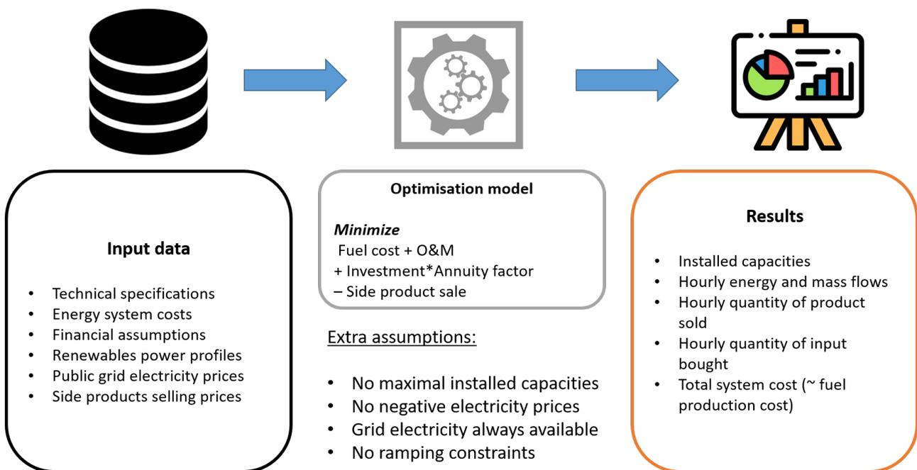
Figure 1: Overview of the OptiPlant optimization model [2]
