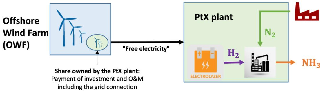
**Figure 3:** Scheme showing a simplified behind-the-meter (BTM) power supply configuration of the Power-to-X plant considered in the model for the large-scale study [2].
